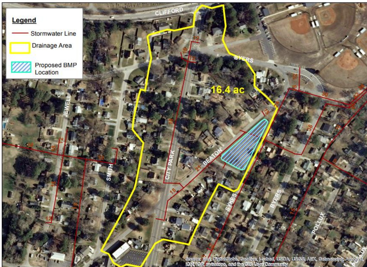
FIGURE 4. BEATON DRIVE LEVEL I WET POND DRAINAGE AREA
