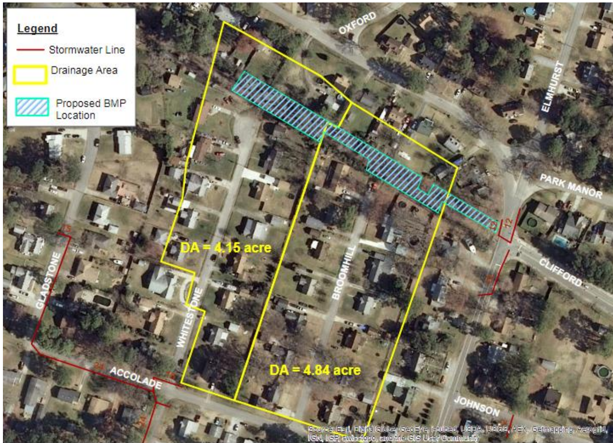
FIGURE 3. CHURCHLAND WET SWALE RETROFIT DRAINAGE AREA
