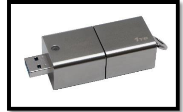
Figure 1 - A 1 terabyte USB storage device measuring 2.8" x 1.1" x 0.8"
